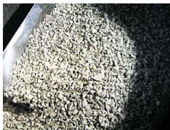
ABS plastic assorted and fractured
