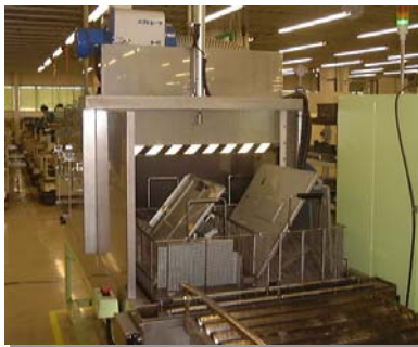
Automatic shower washer that cleans accessories
